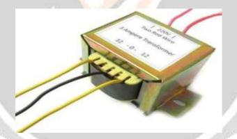
The transformer is a static electrical device that transfers energy by inductive coupling between its winding circuits. A varying current in the primary winding creates a varying magnetic flux in the transformer's core and thus a varying magnetic flux through the secondary winding. 12-0-12 volts 3Amp Center Tapped Step Down Transformer is a general purpose chassis mounting mainstransformer.
